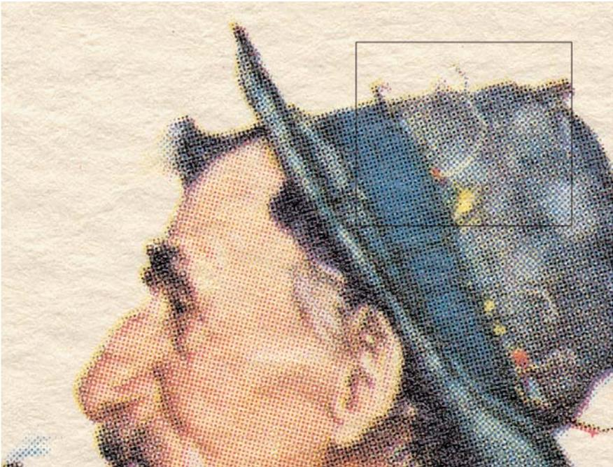
*This is an example of a standard "litho" print using the 4 color print. This process uses a dot screen of cyan, magenta, yellow and black to make up all colors. The problem with this process is that the color screens were hard to register and were visible to the naked eye. A "moire" pattern due to mis-registration is seen here.*
